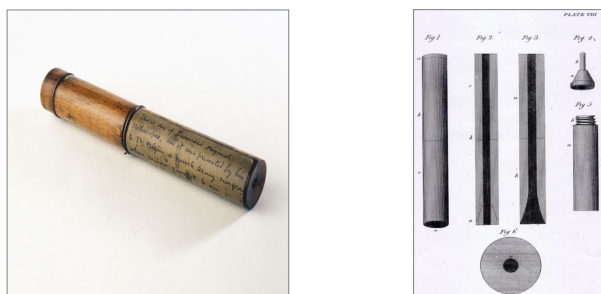
Figure 3–4.: Stethoscope of Laennec from the heroic age, and its cross section illustrated by J. Kergaradec
